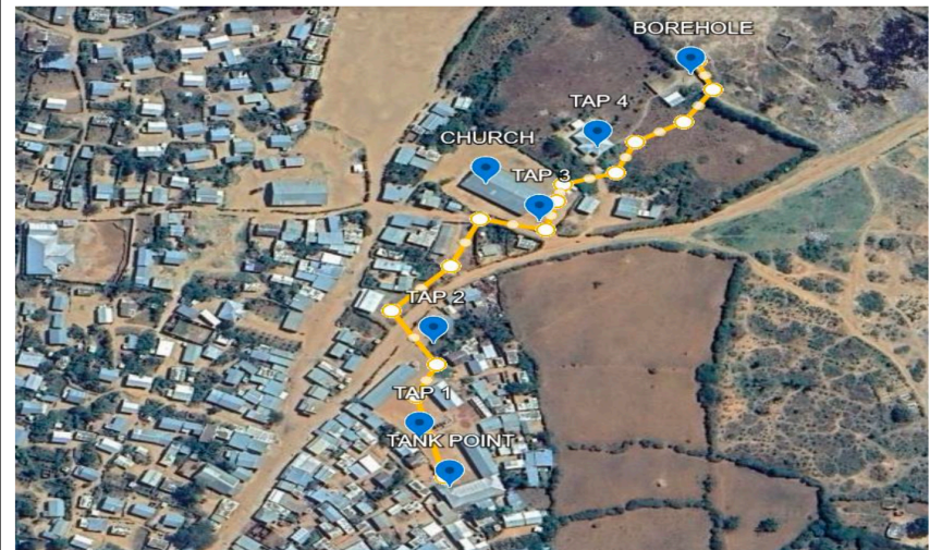
Google earth photo showing the transmission pipe network and the different tap locations
